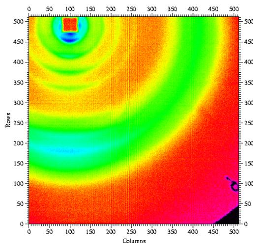
Fig. 2: 2D-detector image of a tristearin dispersion containing 15% w/w lipid matrix. The scattering intensities do not exhibit rotation-symmetrical distribution due to the texture phenomenon in the sample (cf. text).
