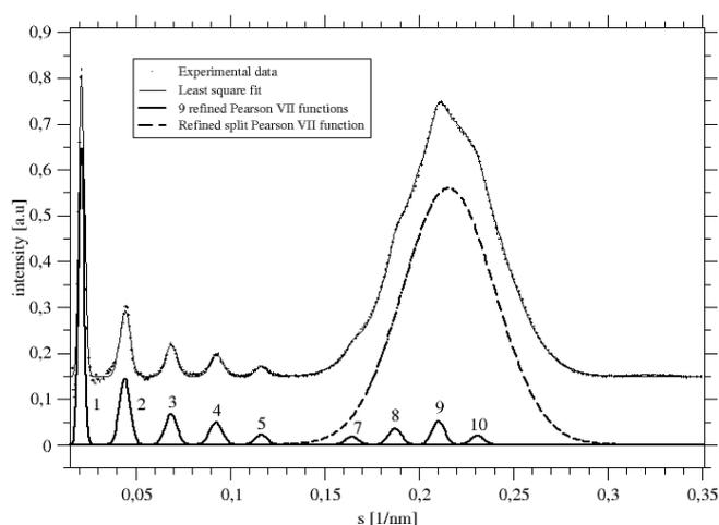
Fig. 1: SAXS pattern of a tristearin dispersion (10% w/w). The pattern was background corrected and fitted to a combination of Pearson VII functions representing the (001)-Bragg reflection of the triglyceride  $\beta$ -modification and the 1<sup>st</sup> to 10<sup>th</sup> order interference due to the lamellar particle arrangement. The experimental data and the least square fit are shifted vertically for better visualization.
