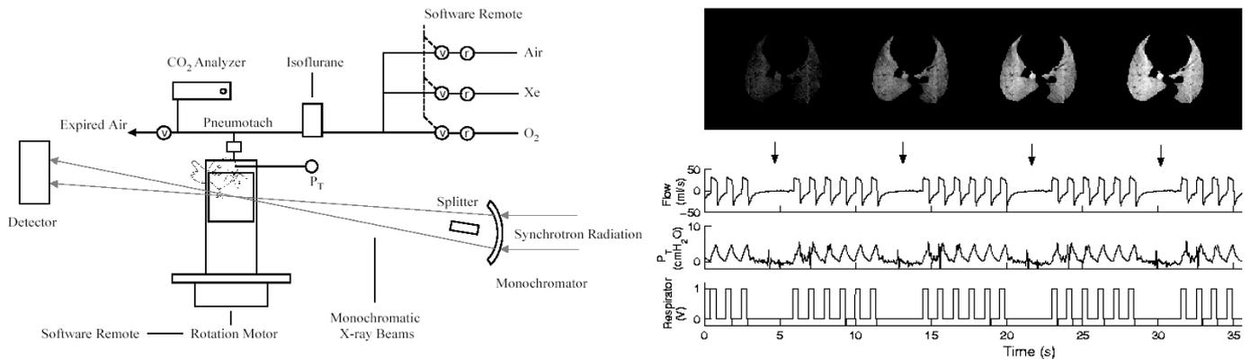
Fig. 2. *Left:* Experimental set-up for mechanical ventilation and CT imaging. A single solenoid valve (v) controls respiration, and three valves are used to switch from one inspired gas mixture to another. *Right:* The sequence of gas flow, tracheal pressure, and opening the respiration valve are shown together with a series of CT images in the wash-in phase.
