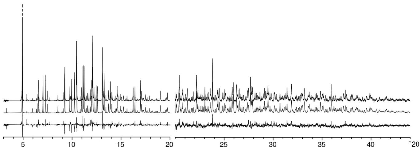
Figure 2. The observed (top), calculated (middle) and difference (bottom) profiles for the Rietveld refinement of the structure of the aluminophosphate MDAP-3. The first peak has been cut at 1/3 of its full height and the second half of the profile has been scaled up by a factor of 6 to show more detail.
