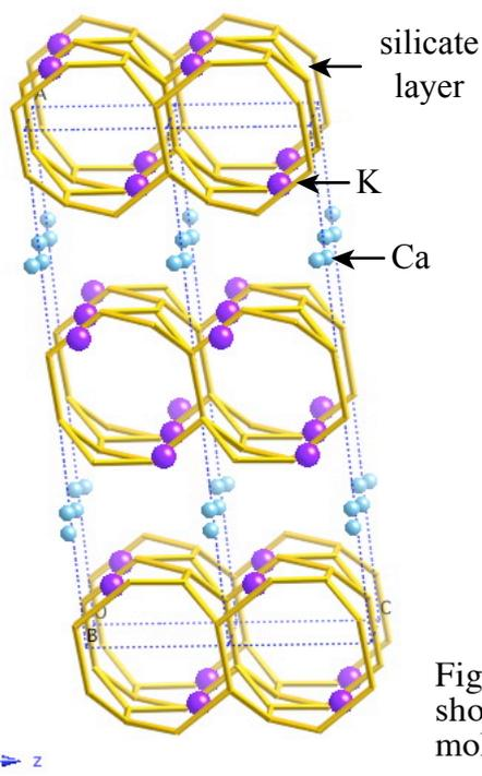
The basic structure of CAS-1 ( $C2$ ,  $a = 24.158 \text{ \AA}$ ,  $b = 7.016 \text{ \AA}$ ,  $c = 6.482 \text{ \AA}$ ,  $\beta = 95.19^\circ$ ) was solved from data collected on a textured sample (ESRF experiment CH-1318), but high-resolution data were needed to complete and refine the structure (Figure 1). Such data had been collected in a previous experiment (01-01-265, December 2002), but the intensities proved to be distorted by an unexpected
