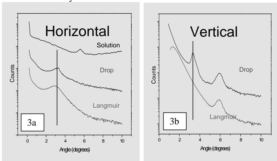
Figure 3 shows the GISAXS scattering in both the in-plane (Fig 3a) and out-of-plane (Fig 3b) directions. Some differences are visible, in particular the in-plane peak appears broader in the langmuir deposition method, whilst it is absent in the vertical scattering. These results are consistent with the transfer of a single layer to the sample, where there is no stacking normal to the surface and therefore no scattering. The broad in-plane peak may be due to the layer being non-close
