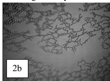
layer to a disordered multilayer structure. Figure 2 indicates the domain structure present in the layer, at the micron scale. The structure in Figure 2a indicates that prior to compression, the particles all appear in bands in one layer, whilst after a full compression-expansion cycle they have aggregated into permanent fractal like branches (Figure 2b). We believe this to be the
