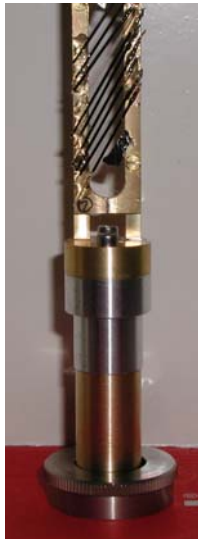
Figure 1: The sample holder and the adapter mountable to the diffractometer tip in the center of Fig. 2 is shown. Filled sample tubes are glued on a frame in the upper part of the holder.
