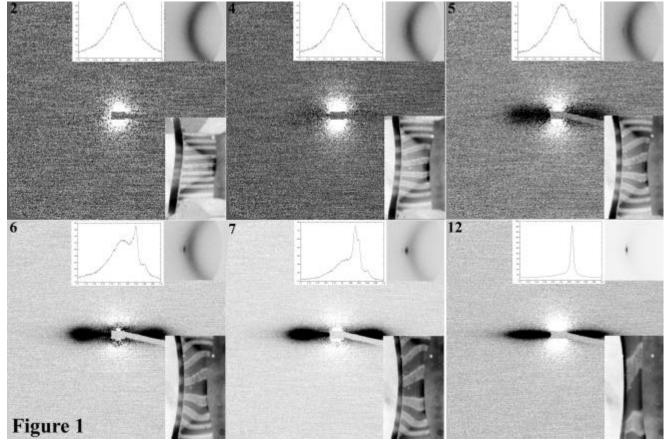
experiments at various temperatures and strains we have established that the structural changes from orthorombic to hexagonal can be achieved either by increasing the strain or by increasing the temperature above ~155°C. The temperature induced structural changes are completely reversible between orthorombic (up to  $155^{\circ}$ C), hexagonal ( up to  $160^{\circ}$ C ) and amorphous ( above  $160^{\circ}$ C ).
