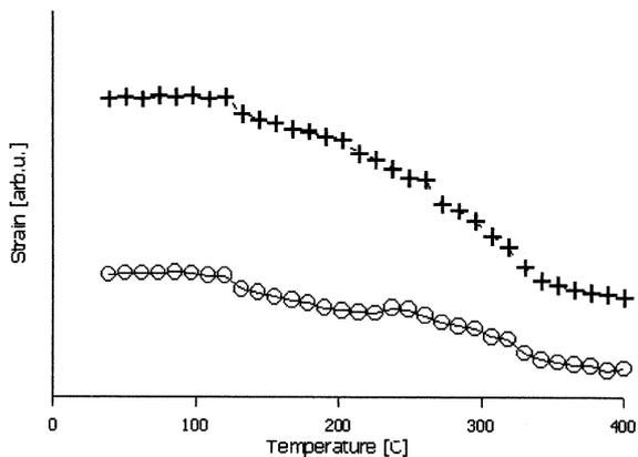
Fig. 2. Plot of strain changes in course of heating from 25° C to 400° C of  $\text{Al}_x\text{Ga}_{1-x}\text{As}/\text{GaAs}$  with  $x=0.3$  implanted with 170 keV He<sup>+</sup> ions to the dose  $3 \times 10^{16} \text{ cm}^{-2}$  presenting the strain in mostly deformed layer (crosses) and the strain close to the surface (circles).
