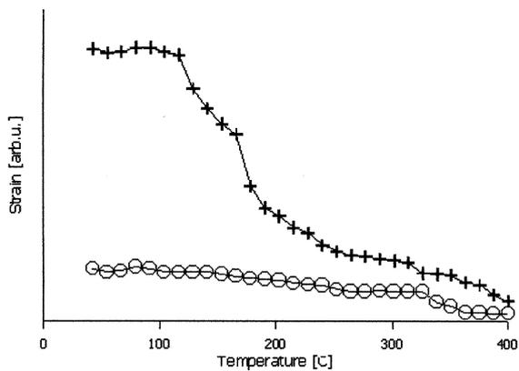
Fig. 1. Plot of strain changes in course of heating from 25° C to 400° C of GaAs implanted with 90 keV H<sup>+</sup> ions to the dose  $3 \times 10^{16} \text{ cm}^{-2}$  presenting the strain in mostly deformed layer (crosses) and the strain close to the surface (circles).
