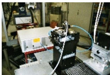
UV-Vis measurements using optical fibres (blue), perpendicular to ED-XAFS measurements
