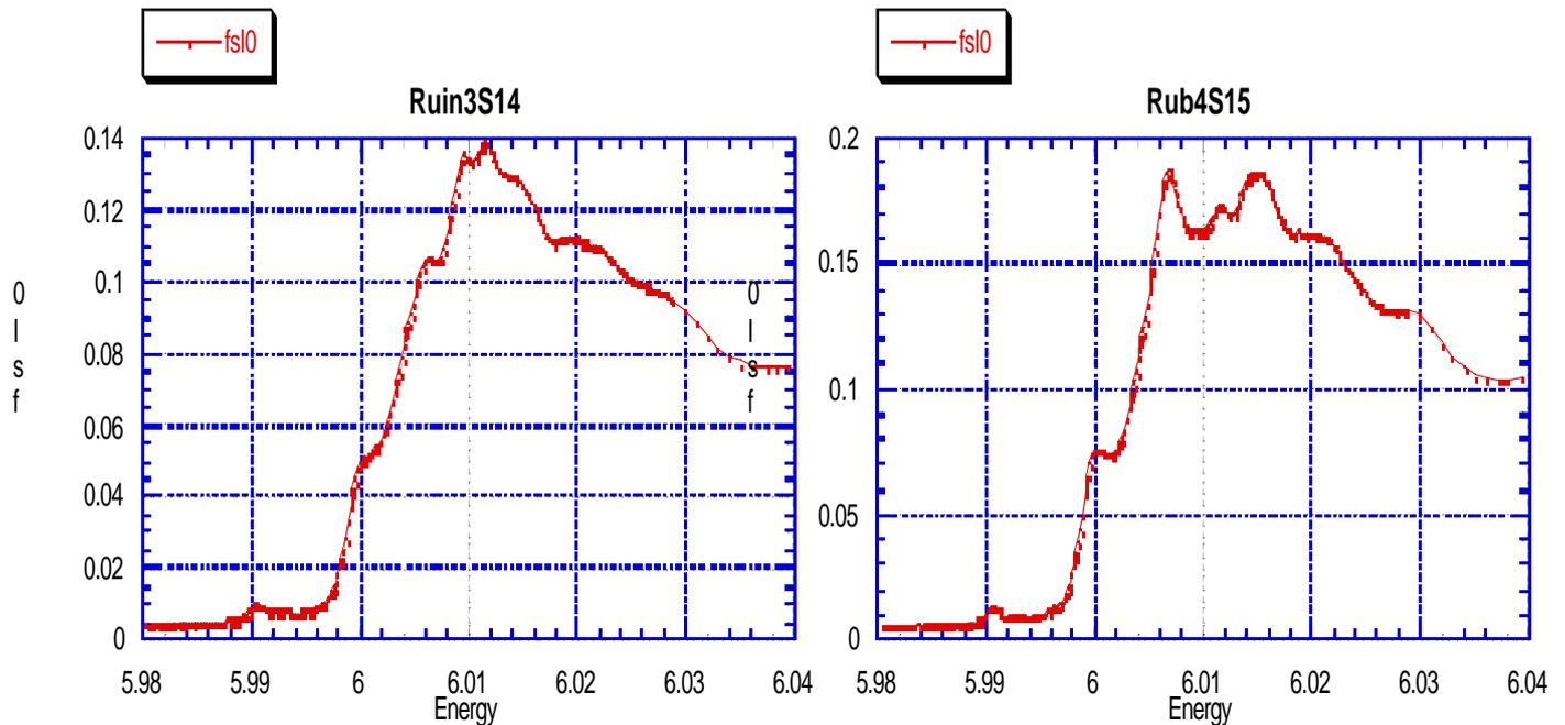
Fig. 1. High resolution Cr K-edge XANES spectra measured on a non-treated ruby (right, denoted by Rub4S15) and an irradiated ruby (left, denoted by Ruin3S14). The high resolution polarised XANES spectra were collected with the plane polarization parallel to the pinnacoidal [0001] face with fluorescence detection at room temperature.
