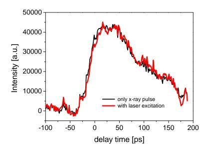
Fig 2: Traces of the scattering from 60nm gold particles supported on a silicon wafer as function of time. There is a slight change in scattering after the laser impact on the particles (delay time 0), which may reflect the lattice disturbance.
