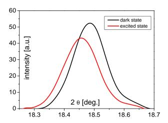
Fig. 1. Debye Scherrer profiles as derived from conventional pump-probe scattering, where the excited state from 60nm gold particles is characterized by a lattice expansion of about 0.15%. In scattering with polychromatic light of 3 keV bandwidth at 15.6 keV peak this profile is smeared out. The working point of the streak camera is at the rising edge of the dark state profile, at about 18.45 degrees for highest sensitivity to lattice changes.
