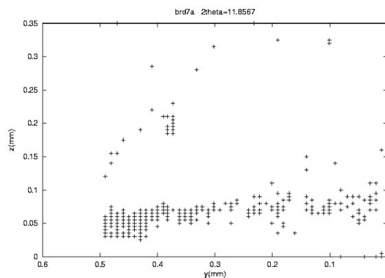
**Figure three:** Spatial distribution plot of diffracted peaks from NiSn intermetallic
