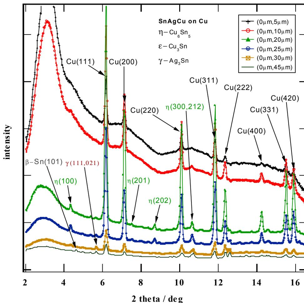
**Figure one:** 1-dimensional XRD peaks from the interface region of a SnAgCu alloy soldered onto a Cu pad. Comparisons between the measured 2-theta values and ones from the Joint Committee of Powder Diffraction Standards (JCPDS) allowed positive identification of the present phases.
