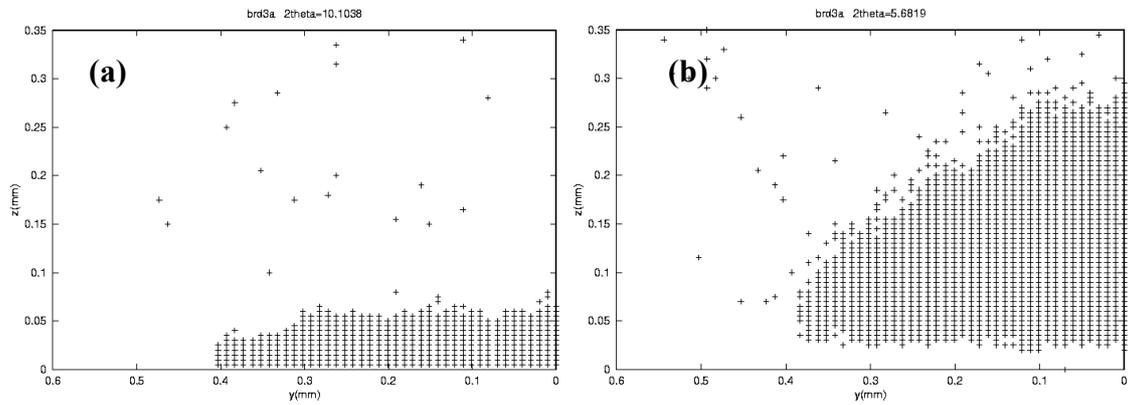
**Figure two:** Spatial distribution plots of diffracted peaks from: **(a)** eta-Tin Copper phase **(b)** gamma-Tin Silver phase. It can be clearly seen that the eta phase is confined to the Cu interface region whilst the gamma phase is present throughout the bulk.
