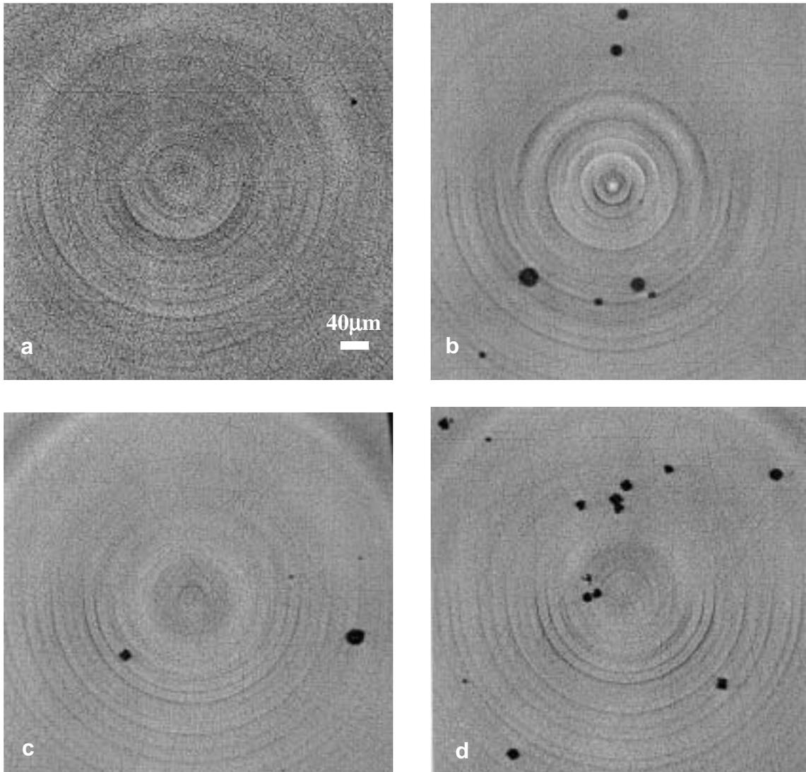
Fig.1. Tomography images of undeformed and creep deformed superalloys
