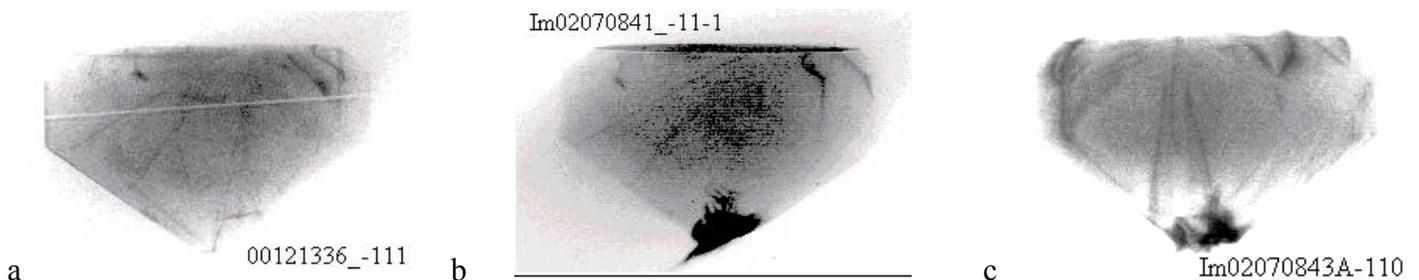
**Figure 1:** Diamond D57 : (a) before high pressure operating, numerous dislocations emerging from a central defect. (b) and (c) broken at 70 GPa, main fracture plane follows a preexisting dislocation.
