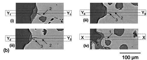
Figure 2: Tomographic sections of arrested short fatigue cracks, showing nucleation as stage I crystallographic cracks.
