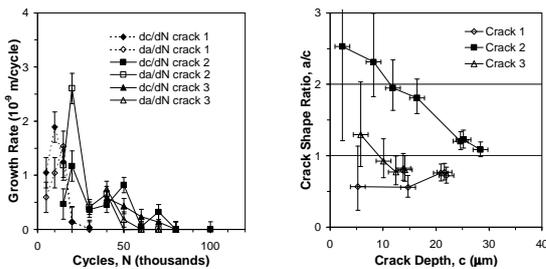
Figure 3: The first quantitative measurement of crack propagation rate and development of crack shape in 3D. Crack depth (c) crack surface length (2a)
