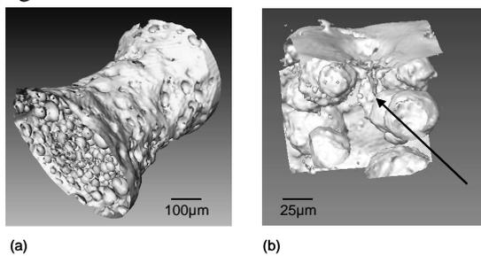
Figure 1: Short fatigue crack nucleus
