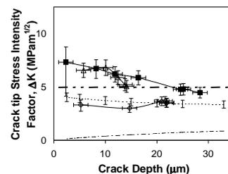
Figure 4: Calculation of crack tip stress intensity factor ( $\Delta K$ ) with increasing crack length in the decreasing stress field of the pore. Crack arrest occurs close to the closure free threshold for long cracks..
