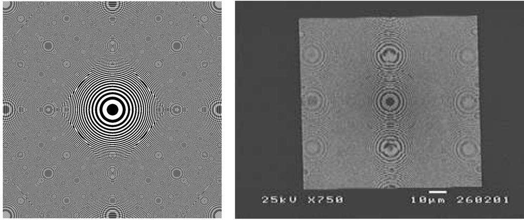
Fig.1: Theoretical modeling of a zone plate pattern for generating a 2 spots beam and the real optical element in tilted view imaged by SEM techniques
