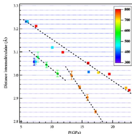
**Figure 3:** Evolution of the first neighbor distance with pressure; circle: experiment; square: simulation. The dashed line is a guide for the eyes.
