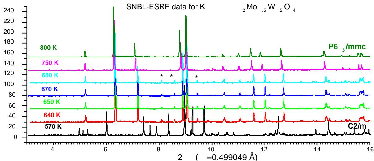
*Figure 3 - Diffraction pattern for the  $K_2Mo_{0.5}W_{0.5}O_4$  at different temperatures.*
