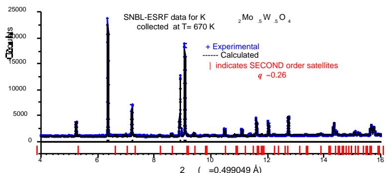
Figure 2 - Diffraction pattern obtained in successive heating-cooling cycles. Evidence of symmetry change
