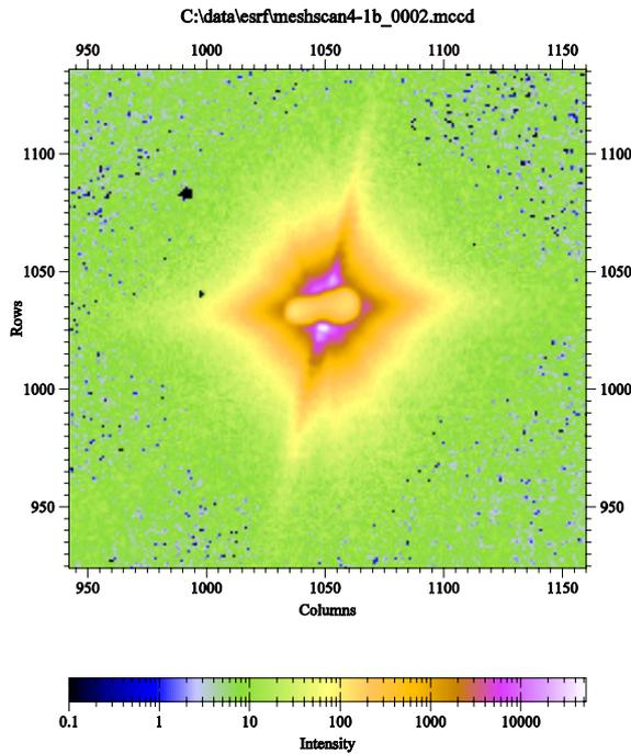
Figure 3: single streaks on a diamond-shaped scattering image (intensity displayed in log).
