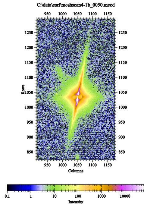
Fig. 4: The intense scattering image (log) reveals large streaks which points to scattering off the narrow crack (0.6,0.3) (very close to the crack-tip) or a tiny crack inside the material.
