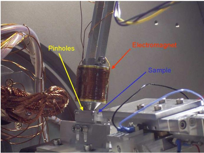
Fig. 1: The experimental set-up in the 4th run of the LTP.
