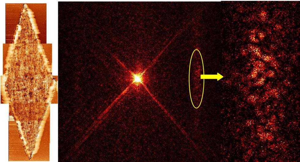
*Fig. 4: The 10x40  $\mu\text{m}$  diamond shape lithographed in FePd thin film and the corresponding SXRMS spectrum using coherent, circular polarisation. The magnetic satellite (in yellow circle and enlargement) shows the typical speckle pattern.*
