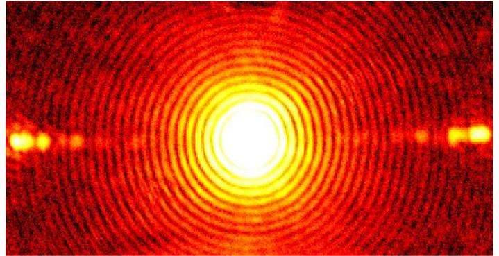
Fig. 2: Specular reflection of the beam. The pinhole results in Airy rings, which show a high coherence of the incident x-ray beam.
