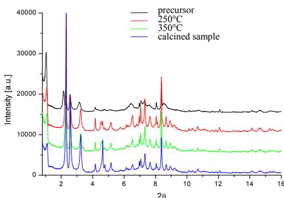
Figure 1: XRD patterns of MCM-22 samples
