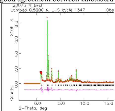
Figure 4: Rietveld analysis of the calcined samples in vacuum
