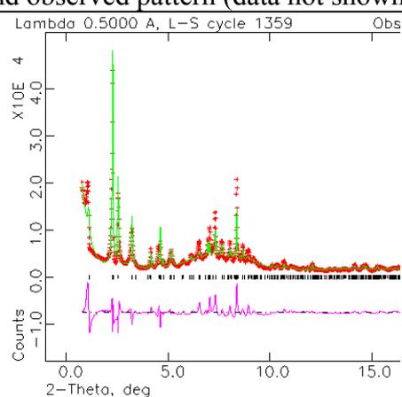
Figure 5: Rietveld analysis of calcined MCM-22 in air.
