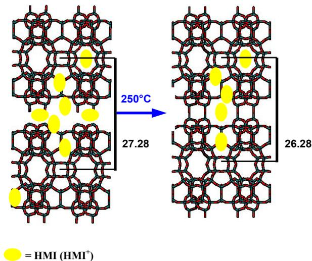
Figure 3: Structural modification during MCM-22 calcination
