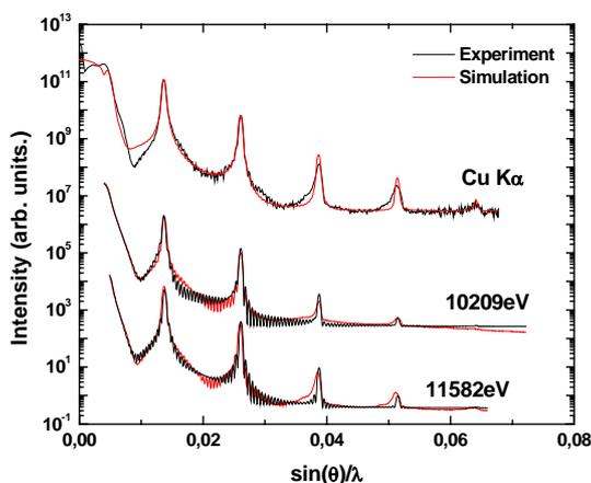
*Fig. 1: Resonant x-ray reflectivity (black curve) performed with Cu K $\alpha$  source and close to the W  $L_{2,3}$  edges. Simulation (red curve).*
