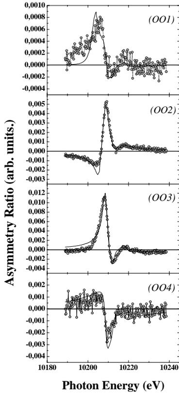
Fig. 3: Energy dependence of the asymmetry ratio  $R$  measured at the four first low order Bragg peaks at the W  $L_3$  edge. Experimental results (open circles) and calculation (drawn lines) leading to the magnetic profile.
