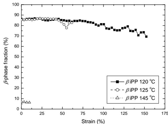
Figure 3. Figure 8: Variation in  $\beta$ -phase fraction with deformation between  $\beta$ iPP samples
