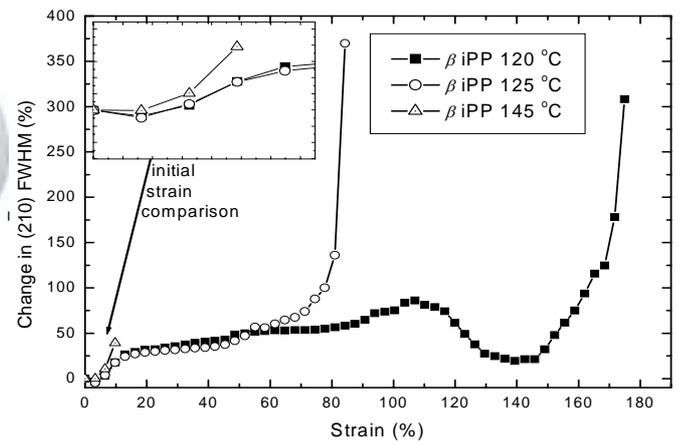
Figure 2. Percentage change during deformation in FWHM of the  $(2\bar{1}0)$  reflection
