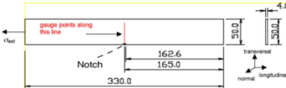
*Fig.1 - Geometry of the investigated samples; the definition of principal axes and the location of gauge points in the neutron diffraction experiments are also shown.*
