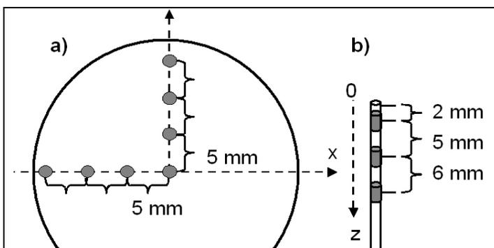
Figure 1 – ROI schematic positioning: a) planform view, showing the cylindrical samples positioning within the FGMMC dowel; samples were extracted at positions echeloned along two perpendicular axes  $\overline{Ox}$  and  $\overline{Oy}$ ; the longitudinal axis of each sample was parallel to the longitudinal axis of the corresponding dowel; b) ROI positioning along the longitudinal axis of each cylindrical sample; scanned ROIs were located at 2, 7 and 13 mm from the SiC-rich end of each sample.
