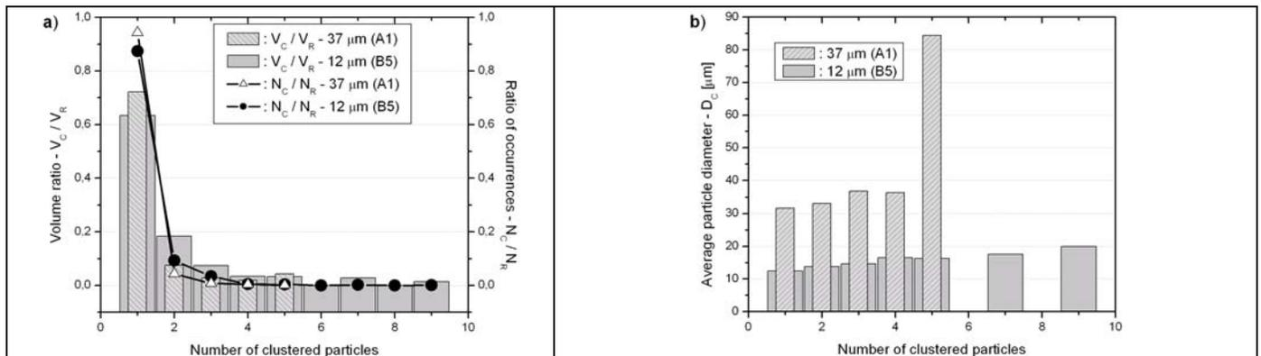
Figure 3 – Particle size effects on: a) volume ratio of clustered particles vs. overall particle volume –  $V_C / V_R$  – and ratio of occurrences of clustered particles vs. overall particle number –  $N_C / N_R$ ; b) average particle diameter,  $D_C$ . In both graphs, the mention to “single-particle” clusters constitutes an expedient way to compute the number of isolated, non-contacting particles (at least up to the precision of the separation algorithm). [12]
