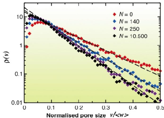
**Fig. 2: Evolution of the volume distribution of the pores for  $\Gamma = 3.0$  at different stages of the compaction.**
