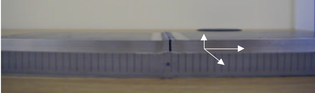
Fig 1. Stress free reference sample (comb) machined from the weld.
