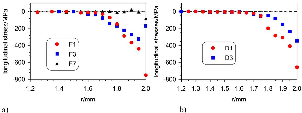
Fig.1: Typical longitudinal stress profiles for samples with a fully lamellar (F) and duplex (D) microstructure. F1, D1 = as-machined, F3, D3 = annealed, F7 = electropolished).
