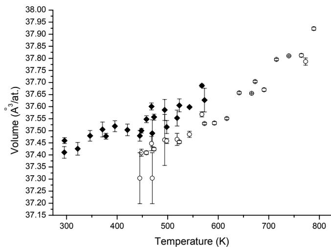
Fig. 2. Temperature dependence of the atomic volume of La metal. Diamonds – dhcp phase; circles – fcc phase.
