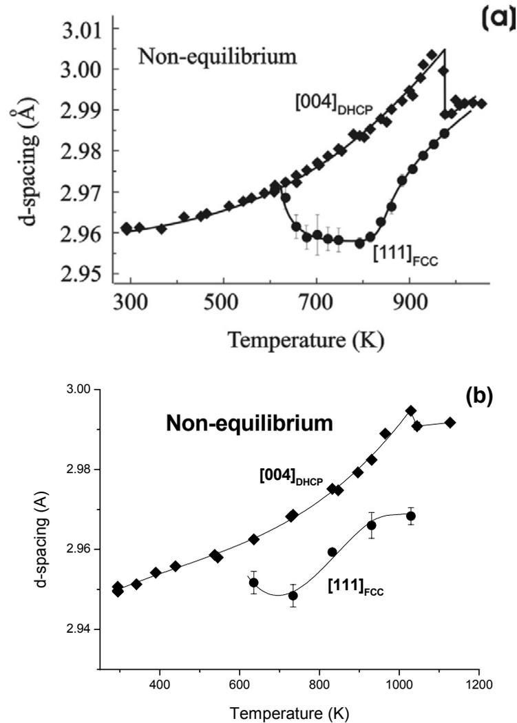
Fig. 1. Linear thermal expansion of (a) Pr and (b) Nd metals. Diamonds correspond to the dhcp phase, and circles to the fcc phase. The interlayer spacing  $d_{[111]c}$  between close-packed layers in cubic phase is compared with its hexagonal analog  $d_{[004]c}$ .
