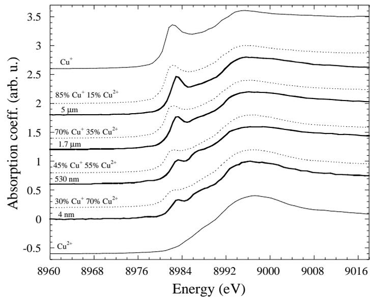
Cu K-edge absorption coefficient spectra collected at different incidence angle (solid line) and compared to that of copper in glass with state of valence (1+) and (2+), respectively indicated as Cu(+) and Cu(2+). Together with the experimental data, the simulation of spectra are also reported (dashed lines). The simulation is made by a linear combination of Cu(+) and Cu(2+).
