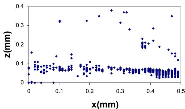
**Figure 2:** Distribution plot of intermetallics in a Pb-free solder bump.
