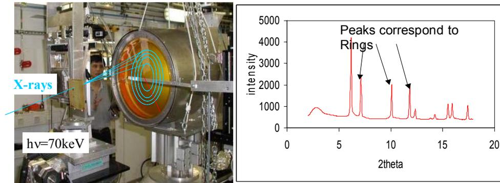
**Figure 1:** Experimental configuration for XRD on ID11 and an example of a ‘caked’ 1D diffraction pattern.
