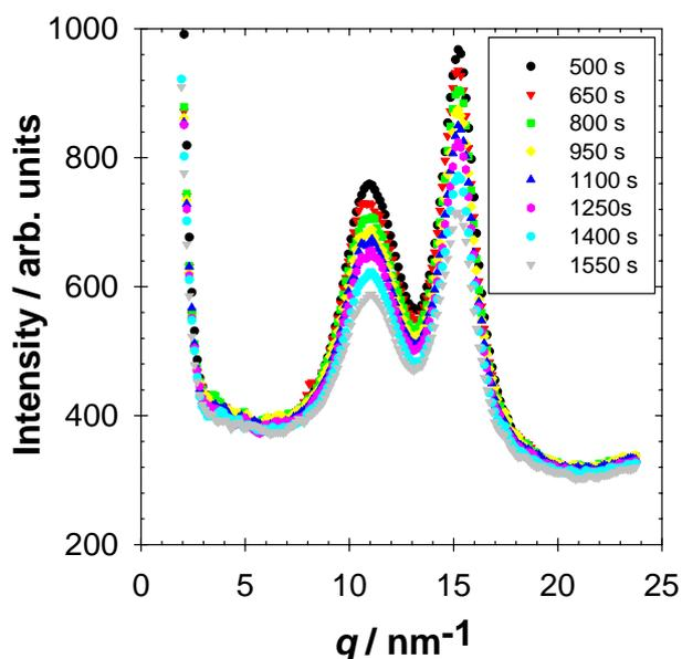
**Figure 3:** Series of scattering profiles of wood at a temperature of 250°C. The data correspond to the third row in Figure 2 and are chosen to separate radiation damage effects due to specimen heating (every frame has suffered the same time of illumination by the X-ray beam, but an increasing time at  $T=250^\circ\text{C}$ ).
