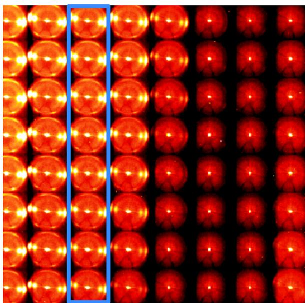
**Figure 2:** Part of a scanning mesh of 2D diffraction patterns from a thin wood section at a temperature of 250°C, beam size:  $\sim 5 \mu\text{m}$ , step:  $10 \mu\text{m}$ . The scan started at the left upper and ended at the right lower corner of the figure by successively scanning line by line. The time between two succeeding frames in a vertical row is 150 s.
