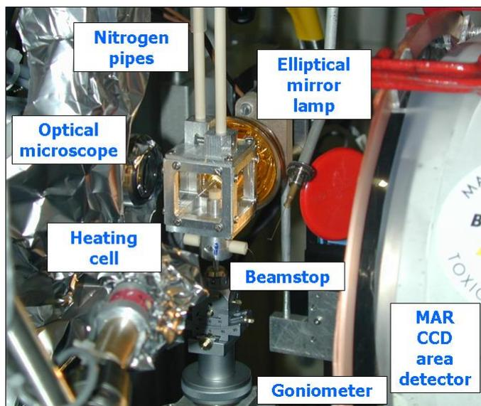
**Figure 1:** Photograph of the experimental setup with the *in-situ* heating cell at the ESRF microfocus beamline ID13.
