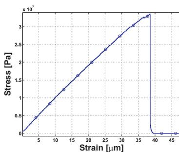
Figure 3. Stress/strain curve of a Norway spruce sample. The circles point out where one measured frame (diffraction pattern) ends. The first frame measured in tension is number 2.
