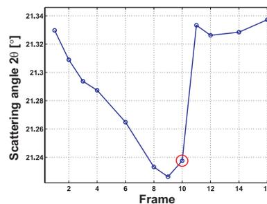
Figure 4. The change in scattering angle of reflection  $004$ . Frame number denotes the position in the stress-strain curve. Approximate position of fracture is indicated by the red circle.
