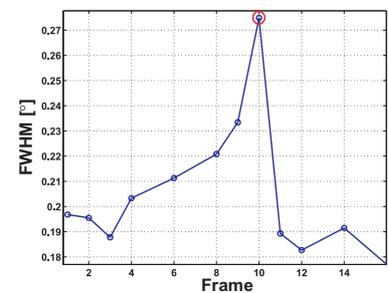
Figure 5. The FWHM of reflection  $004$  in the same direction as in Figure 4. Frame numbers and position of fracture as in Figure 4.
