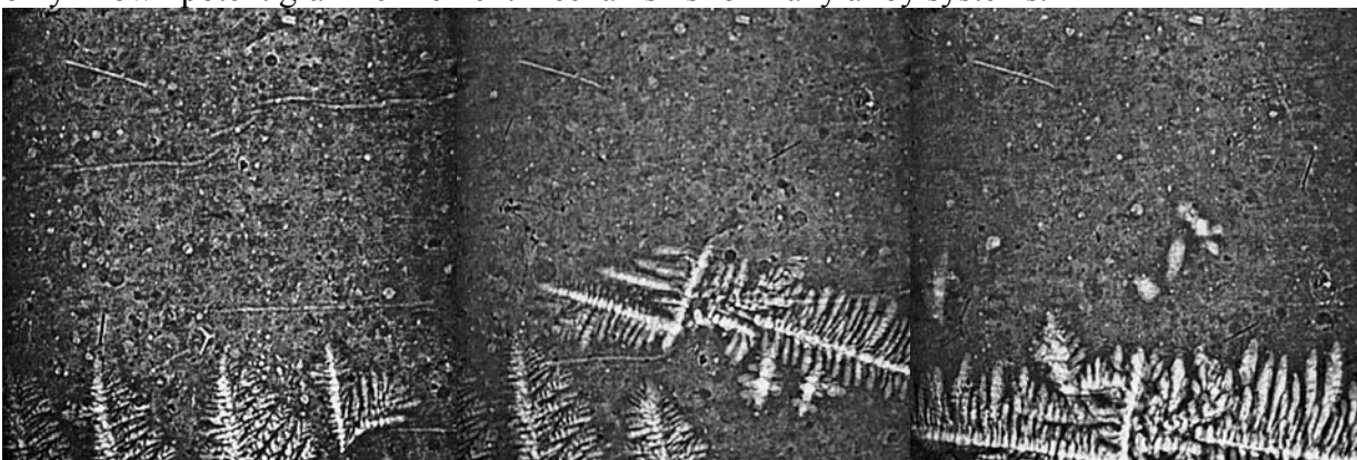
Figure 2. From left to right. 1) Detached ternary branch growing rapidly in the melt. 30 frames (10 s.) later where the fragment has grown to a large crystal preventing further growth of the columnar front. Two other fragments have loosened and coagulated at the colder side of the primary fragment 3) 45 frames (15 s) later: the columnar front has been replaced by the equiaxed crystal, five new fragments have just detached from the new front.
