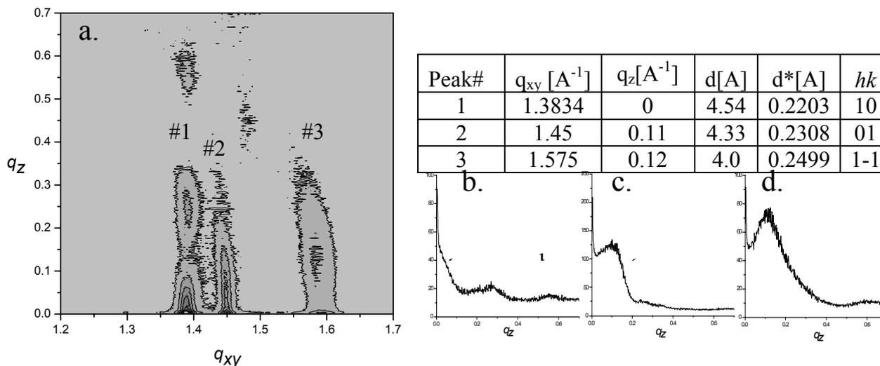
**Figure 1.** (a) Diffraction intensity map of  $q_z$  vs.  $q_{xy}$  obtained in a GIXD experiment from PDA trilayer on air-water interface. (b-d) Bragg rods for the three observed peaks: (b) Bragg rod at  $1.383 \text{ \AA}^{-1}$  (#1). (c) Bragg rod at  $1.450 \text{ \AA}^{-1}$  (#2). (d) Bragg rod at  $1.575 \text{ \AA}^{-1}$  (#3).
