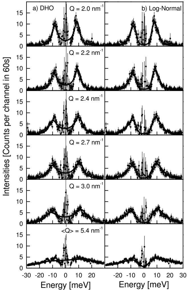
Fig. 1 : fits of the inelastic spectra after subtraction of the freely adjusted elastic contribution at  $Q$ -values ranging from  $2 \text{ nm}^{-1}$  to  $3 \text{ nm}^{-1}$ . The bottom spectra at  $5.4 \text{ nm}^{-1}$  are the sum of data accumulated on analyser 2 at 5, 5.2, 5.4, 5.7 and  $6 \text{ nm}^{-1}$ . (a) DHO fits. (b) Log-Normal fits.
