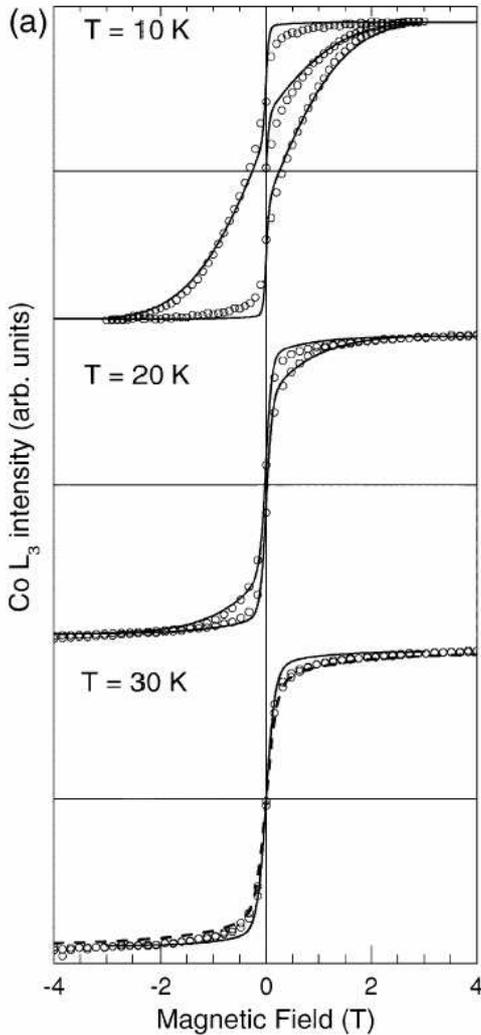
Fig. 2 : XMCD magnetisation curves at the  $L_3$  Co edge as a function of temperature with the magnetic field perpendicular to the sample surface.
