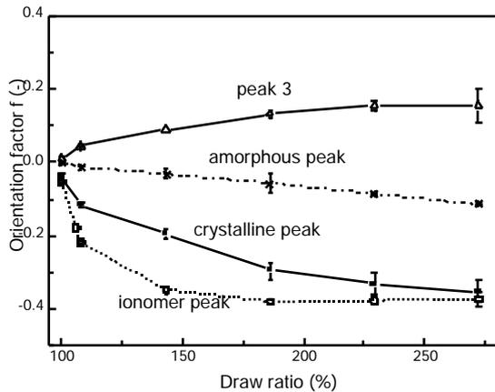
Figure 2 : Orientation factors of the different peaks of Nafion 117 (left) and Nafion 125 (right) as function of draw ratio.
