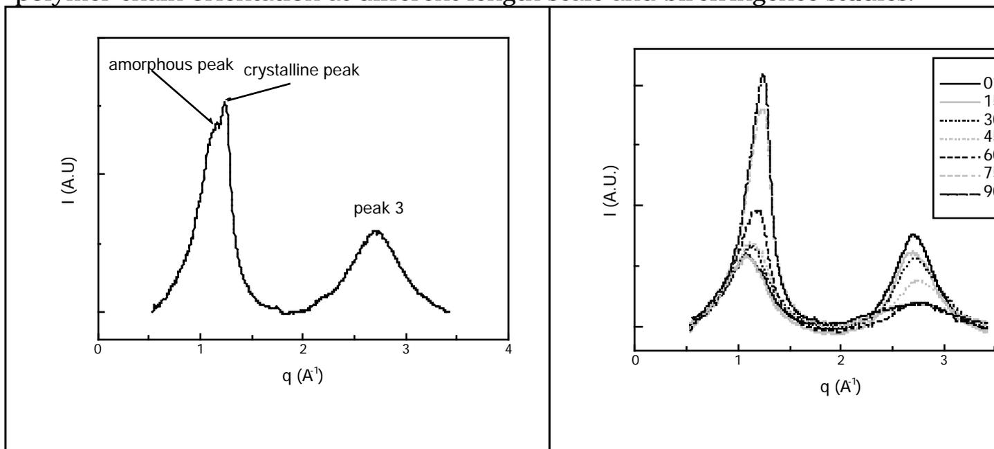
Figure 1: WAXS result Nafion 125: at meridian (left picture) for at DR=100%, and DR=229% for different azimuthal angles (right picture).
