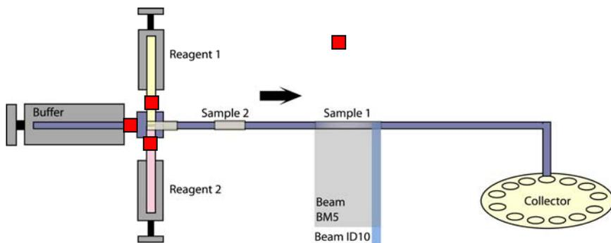
**Figure 1:** The modified stopped flow apparatus. Two separate motors drive the syringes. One motor drives the reagents (1) and (2) for mixing. After waiting for a defined reaction time, the second drive pushes the sample across the beam and then into the collection tube.
