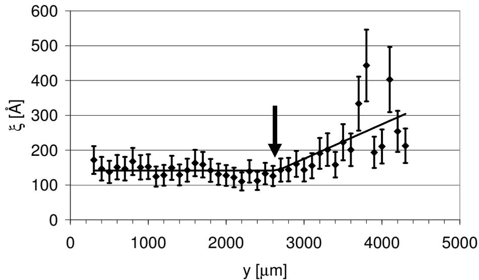
Fig. 1. Most-prominent in-plane length  $\xi_{\max}$  as a function of the scan position. Note the double gradient structure: PS- $\rightarrow$ Ag-layer with  $\xi_{\max} = 142\text{\AA}$  and the second increase around  $y=2600\mu\text{m}$  indicating the end of the influence of the liquid-air-polystyrene boundary conditions.
