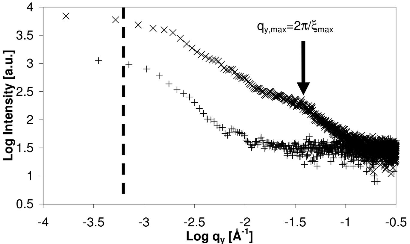
Fig. 2. Out-of-plane scans at  $y=1700\mu\text{m}$  (pure PS-film) and  $y=3100\mu\text{m}$  (Ag-layer) for  $q_z=0.102\text{\AA}^{-1}$ . The side maxima at  $q_{y,\text{max}}$  indicates the most-prominent in-plane length via  $\xi_{\text{max}}=2\pi/q_{y,\text{max}}$  as a result of the build-up of the Ag-cluster layers. The dashed line marks the resolution of the  $\mu\text{GISAXS}$  experiment.
