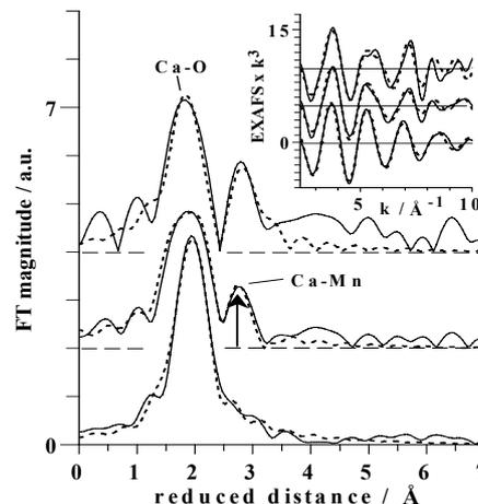
**Figure 3:** FTs of EXAFS spectra (insets) of ~80 Ca / 4 Mn (bottom) and Chelex-treated PSII samples (middle). Top: tentative pure spectrum of Ca bound to the Mn complex. Dashes, simulations (Table 1).
