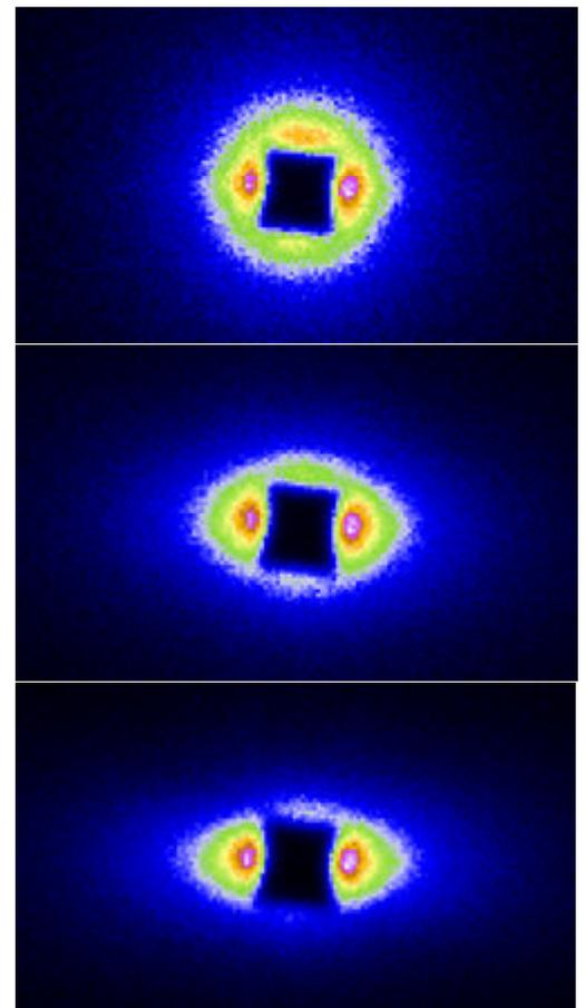
Figure 2. Small Angle X-Ray Scattering 2D images of the Isotropic Gel (upper), Nematic Gel (lower) and the transition zone between these two phases (middle).
