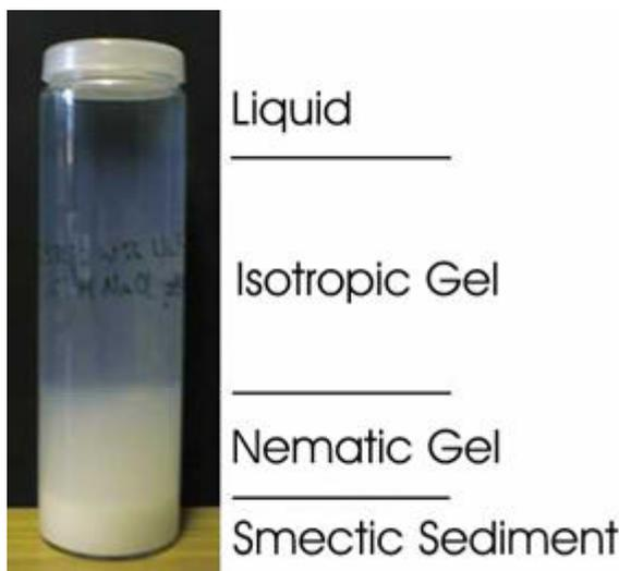
Figure 1. One of our samples showing four strata due to gravitational forces, that effectively sorted the particles by size.
