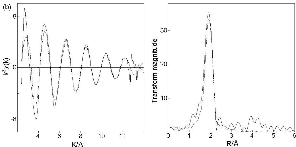
**Fig.1** Experimental (—) and calculated (---) Fourier filtered (1-25) EXAFS and its Fourier Transform for CuZSM-5; (b) calcined ( $k^3$ -weighted).
