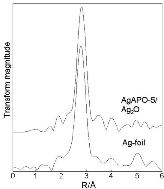
**Fig.3** Experimental Fourier filtered (1-25) EXAFS and its Fourier Transform for as synthesised AgAPO-5 made from silver(I)oxide compared to Ag-foil.
