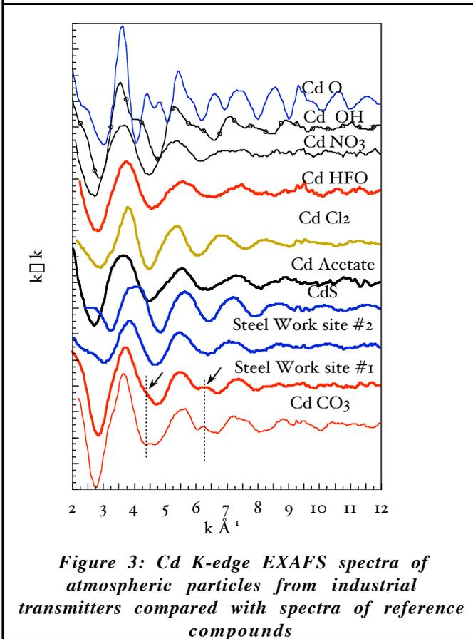
Figure 3: Cd K-edge EXAFS spectra of atmospheric particles from industrial transmitters compared with spectra of reference compounds
