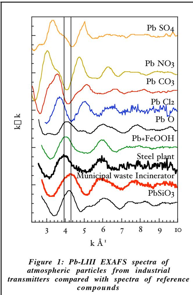
Figure 1: Pb-LIII EXAFS spectra of atmospheric particles from industrial transmitters compared with spectra of reference compounds
