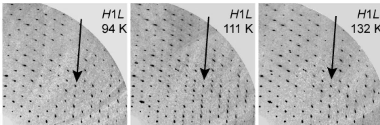
Fig. 2. Reciprocal layers reconstructed from the diffraction intensity. Note the weak superstructure reflections appearing at 111 K, indicating a doubling of the unit cell axis as shown by the arrow.
