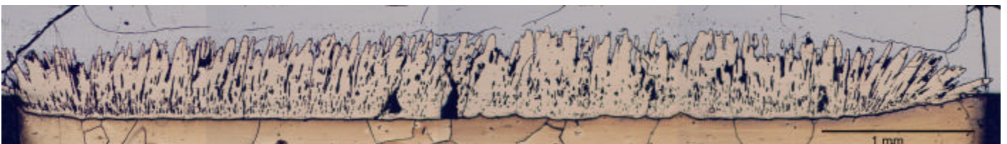
Figure 2 : Conventional observation by metallography and optical microscopy. \theta = 750^{\circ}\text{C} , t = 6 h, diam. = 6mm.
