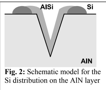
**Fig. 2:** Schematic model for the Si distribution on the AlN layer
