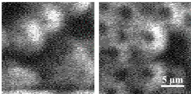
**Fig. 1:** Lateral distribution of Si for a) metal-rich and b) N-rich growth conditions using the integrated intensity of the Si  $K\alpha$  line of the fluorescence spectra.
