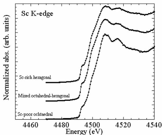
**Figure 2:** Comparison between Sc K-edge  $\mu$ -XANES spectra taken in different phases. The lower spectrum is taken in the Sc-poor while the upper in the Sc-rich phase. The middle spectrum exhibit both coordination
