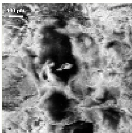
**Figure 1:**  $\mu$ -XRF fluorescence map of Sc  $K\alpha$  intensity on the sample with nominal Sc content  $x=0.28$ , with a resolution of  $5\mu\text{m}$ . The Micron marker is shown
