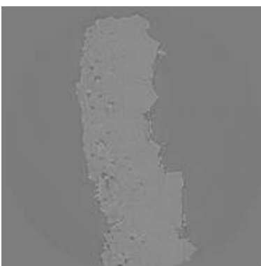
Figure 2a: Slice of a fast reconstructed tomogram of untreated jarosite ( \text{KFe}_3(\text{SO}_4)_2(\text{OH})_6 ); size of the slice 573 \mu\text{m} x 573 \mu\text{m} ; samlpe: (ja200_1__slice.jpg
