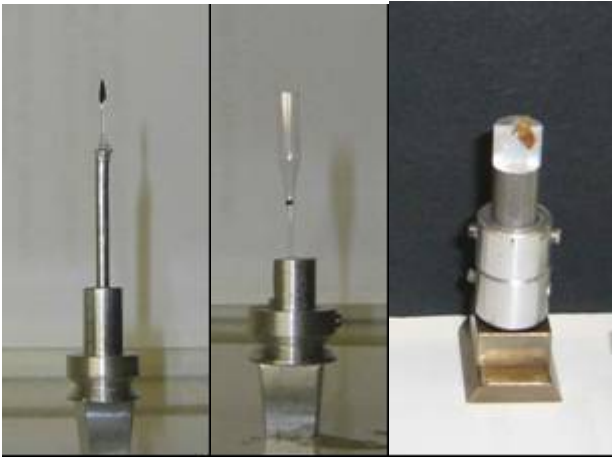
Fig 1a,b,c1: Variants of mounting fragile mineral assemblages
