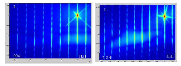
It has been shown on previous samples with larger period  $(0,58\mu\text{m})$  that the secondary diffraction peak appearing for smaller value of L and H (for -2 -2 4 map) is due to an homogeneously Si strained area between the trenches. The strain is negative across the trenches and positive perpendicular to the surface. In this case the homogeneous strain across the trenches is -3.1\*10<sup>-3</sup> and 2.9\*10<sup>-3</sup> vertically.
