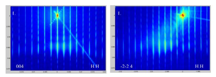
For this sample the homogenous strain would -2.8\*10<sup>-3</sup> horizontally and 3.5\*10<sup>-3</sup> vertically. But on the 004 reciprocal space mapping, there is an asymmetry in the diffraction between positive values of H,H and negative ones. Therefore, a direct measurement of the strain is not possible anymore. Further analyses are in progress to understand this asymmetry: geometry of the lines, anisotropy of process...
