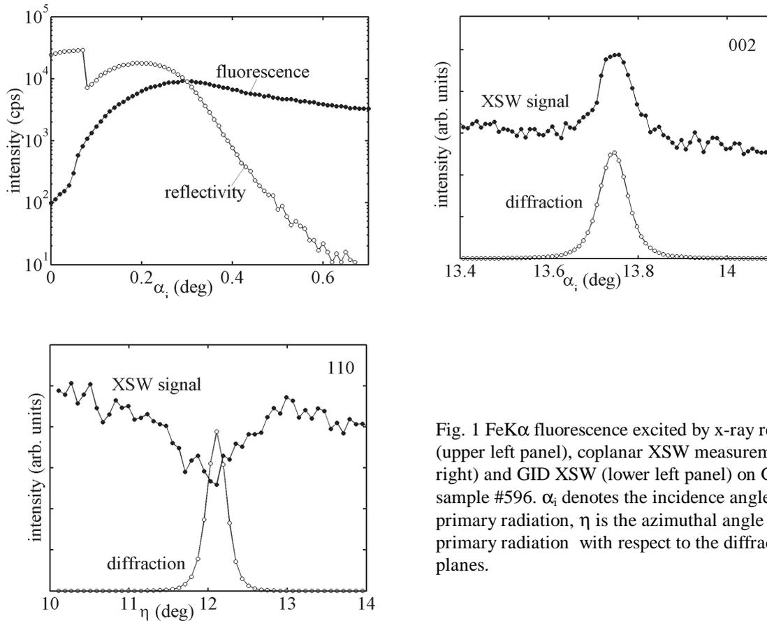
Fig. 1 FeK $\alpha$  fluorescence excited by x-ray reflection (upper left panel), coplanar XSW measurement (upper right) and GID XSW (lower left panel) on GaFeN sample #596.  $\alpha_i$  denotes the incidence angle of the primary radiation,  $\eta$  is the azimuthal angle of the primary radiation with respect to the diffracting net planes.
